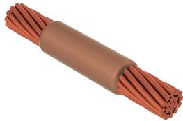
nVent ERICO Cadweld Cathodic Connections are the preferred method of exothermically welding cathodic protection anode leads to pipes (steel or cast iron), tanks, and other structures. Cathodic protection systems are designed to prevent galvanic corrosion along a pipeline or in various structures. nVent ERICO Cadweld Cathodic Connections use a special welding material alloy to minimize heat effect on the steel, which is especially important on thin wall and high stress pipes.
