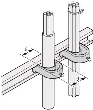
C-Rails are for better cable management. Installation generally behind the 19" uprights. They are compatible with standard cable clabs.
