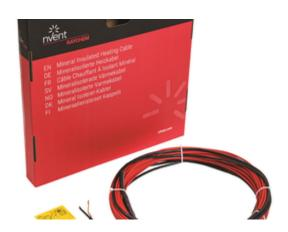
nVent RAYCHEM EM-MI-PACK is a mineral insulated (MI) constant output heating cable used to prevent snow and ice formation on ramps/access ways, with variable power output depending on cable spacing (to 300 W/m²). It can withstand high temperature applications e.g hot poured asphalt followed by mechanical high pressure roller. Pre-terminated.
