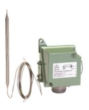
nVent RAYCHEM AMC-1B is a line-sensing thermostat designed to control heat tracing systems in non-hazardous locations. It senses pipe or tank wall temperatures, used to control a single heat tracing circuit or switch multiple circuits with a contactor, it has an adjustable set point. Also used to indicate low temperature or high temperature alarm conditions.
