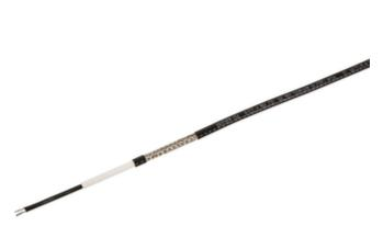
nVent RAYCHEM ETL self-regulating trace heating cables provide energy efficient pipe freeze protection. R-ETL-A/B are suitable for on- or in-pipe applications, R-ETL(-A/B)-CR for on-pipe only. Each are available in two power outputs (10 and 16 W/m at 5 °C), supported by a full range of heat shrinkable connections and accessories.
