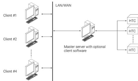
**Figure 2.1.2 Typical single master, multiple client system**
