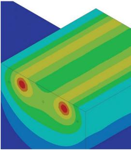
Finite Element Analysis to Rail & Guideway projects helps ensure that sufficient heat is provided for effective snow and ice melt capability.
